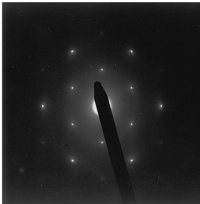
Fig. 3 Typical TEM image and SAED pattern on an Mn-EG particle
